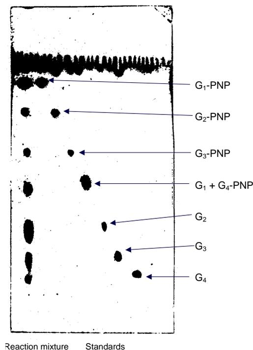
Fig. 3. TLC of reaction mixture of maltotetraose donor and PNP-glycoside acceptor catalysed by Y151M. Eluant:  $\text{CHCl}_3$ :MeOH:water = 8:5:1.
