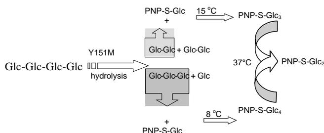
Fig. 6. Schematic representation of the suggested reaction of maltotetraose and PNP 1-S- $\beta$ -Glc catalysed by Y151M.
